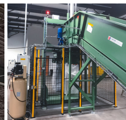
Fence with integrated safety door, ensuring operator safety
